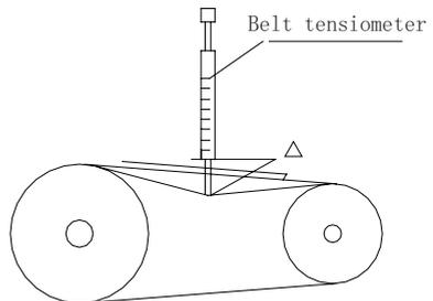
Fig.10.8 Adjust the tightness of the belt Fig. 10.9 Utilization of the belt tensiometer
