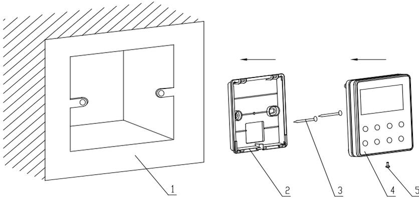
Fig.4.1: Sketch for Installation of Wired Controller
