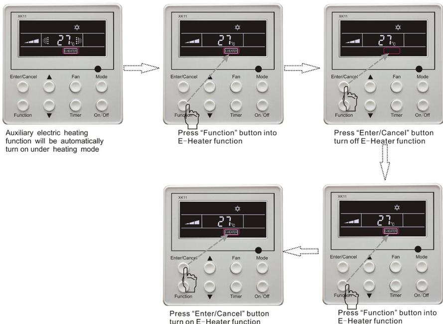
Fig. 5.11 Auxiliary Electric Heating Function Setting
