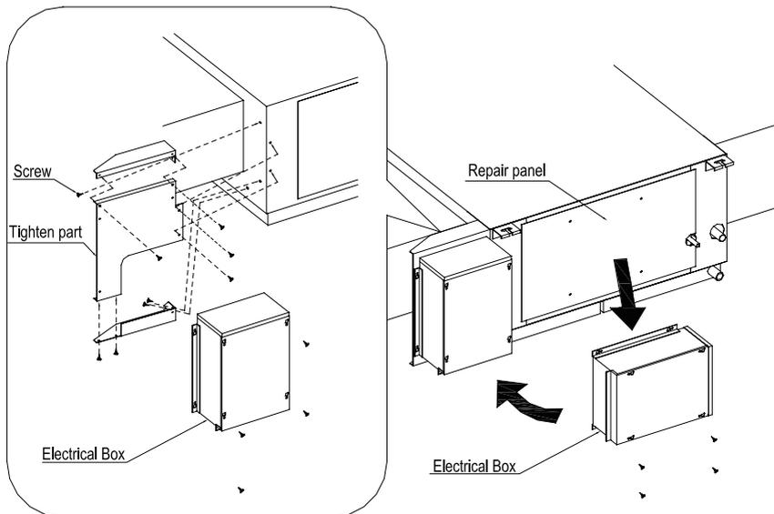
Fig. 10.4 Schematic for the Electrical Box part
