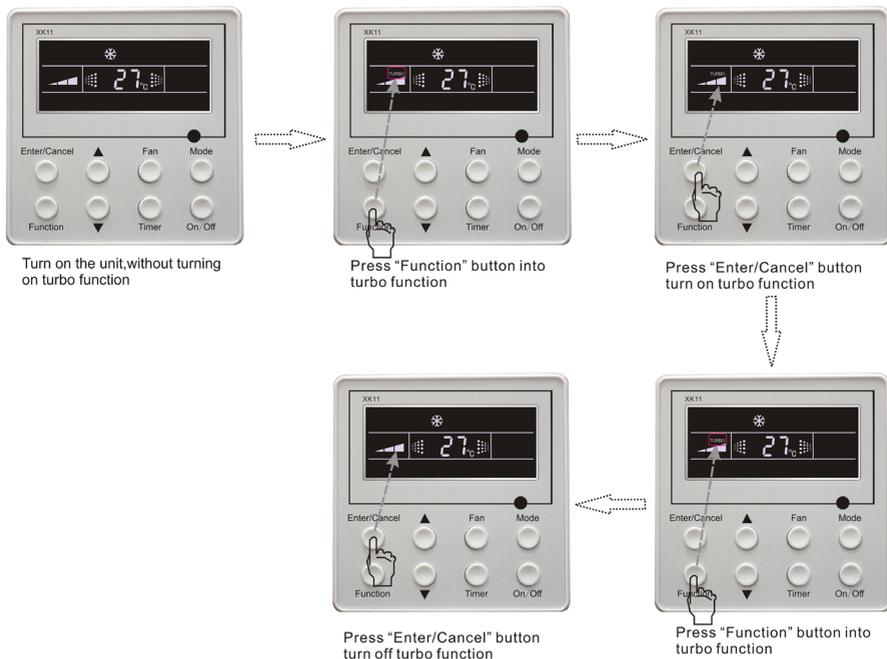
Fig.5.9 Turbo Function Setting
