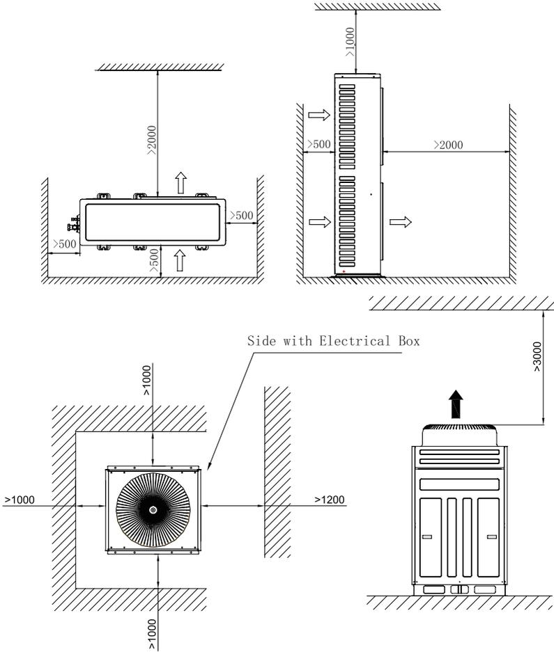
Schematic for the installation of the outdoor unit
