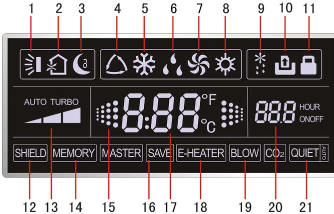
Fig.2.2 LCD display
