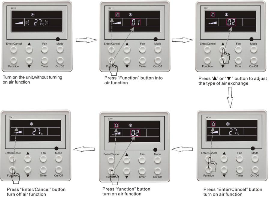
Fig.5.7 Air exchange device
