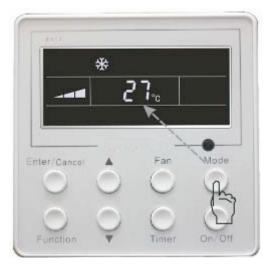
Press ▲ or ▼ button for increase or decrease of setting temperature under on state of the unit. If
