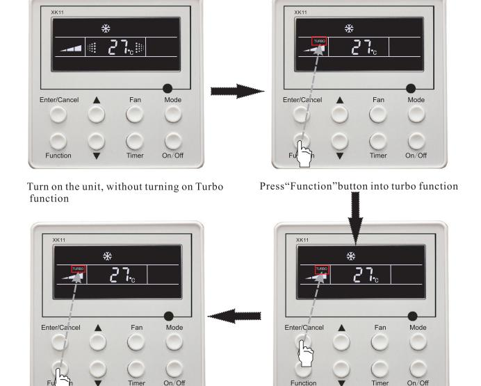
Press"Function"button into turbo function
