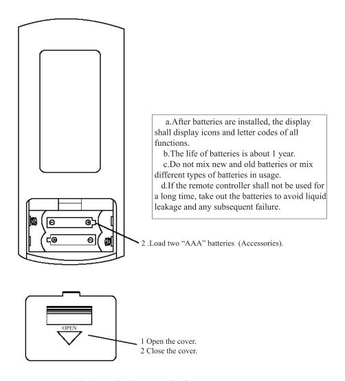
Fig.25 Replacing Batteries for Remote
