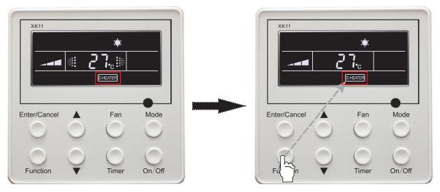
Auxiliary electric heating function will be automatically turn on under heating mode
