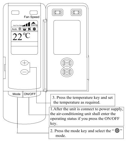
Fig. 22 Heating Mode Operation
