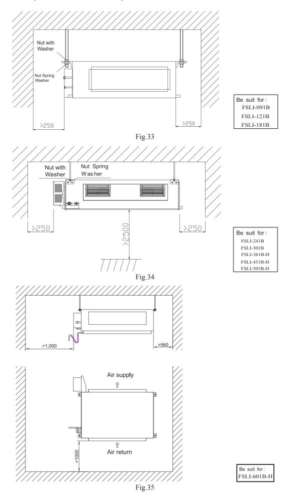
Warning: The height of installation for the indoor unit should be 2.5m above.
