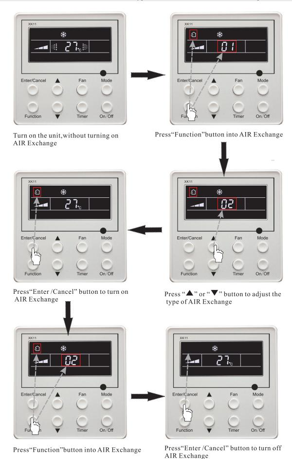
Fig.12 Air exchange device
