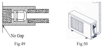
Cautions: After the pipes are wrapped by protective materials, never bend the pipes to form very small angle, and otherwise the pipes may crack or break.
