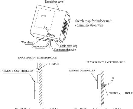
Fig.51 Surface mounting of Cable Fig.52 Concealed mounting of Cable
