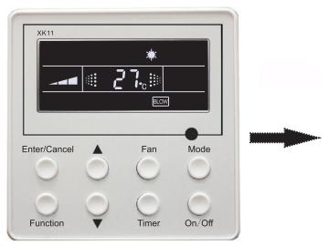
Turn on the unit, without turning on blow function
