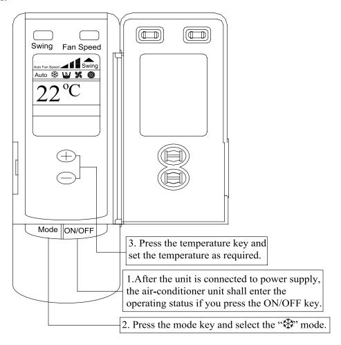
Fig. 21 Cooling Mode Operation
