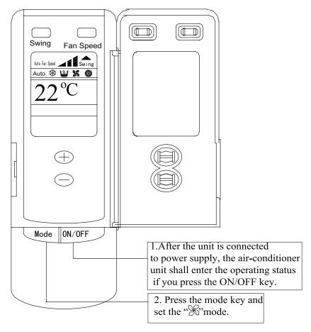
Fig.24 Fan Mode Operation
