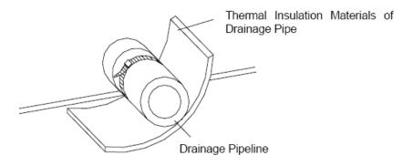
Fig. 43 Thermal Insulation of Drainage Pipeline
