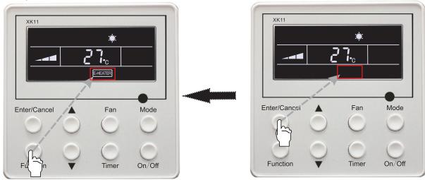
Press"Function"button into E-Heater function
