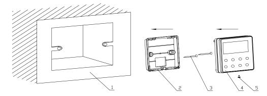
Fig.4 Sketch for Installation of Wired Controller
