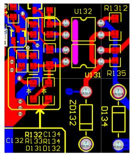
(3) Test the voltage of pin 3 and pin 4 of U131 with universal meter (voltage of both sides of R134). The voltage should be variable. (test 11) Test the voltage of pin 1 and pin 2 of U132 with universal meter (voltage of both sides of C134). The voltage should be variable. (test 12) Otherwise, there is malfunction of mainboard of outdoor unit.
