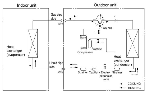
Connection pipe specification: Liquid pipe:1/4" (6mm) Gas pipe:3/8" (9.52mm)
